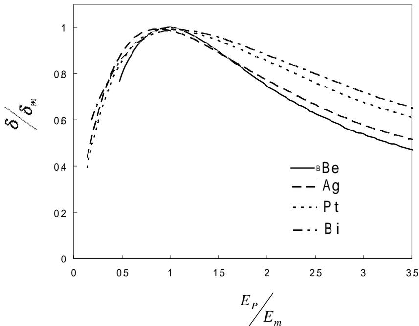
Fig.3 Theoretical universal curve plot as a function of absorption coefficient for Be, Ag, Pt and Bi
