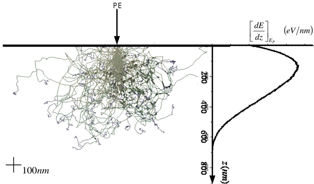
Fig.1 Trajectories of incident electrons of 1keV in a Cu target. The energy dissipation in-depth is also depicted.
