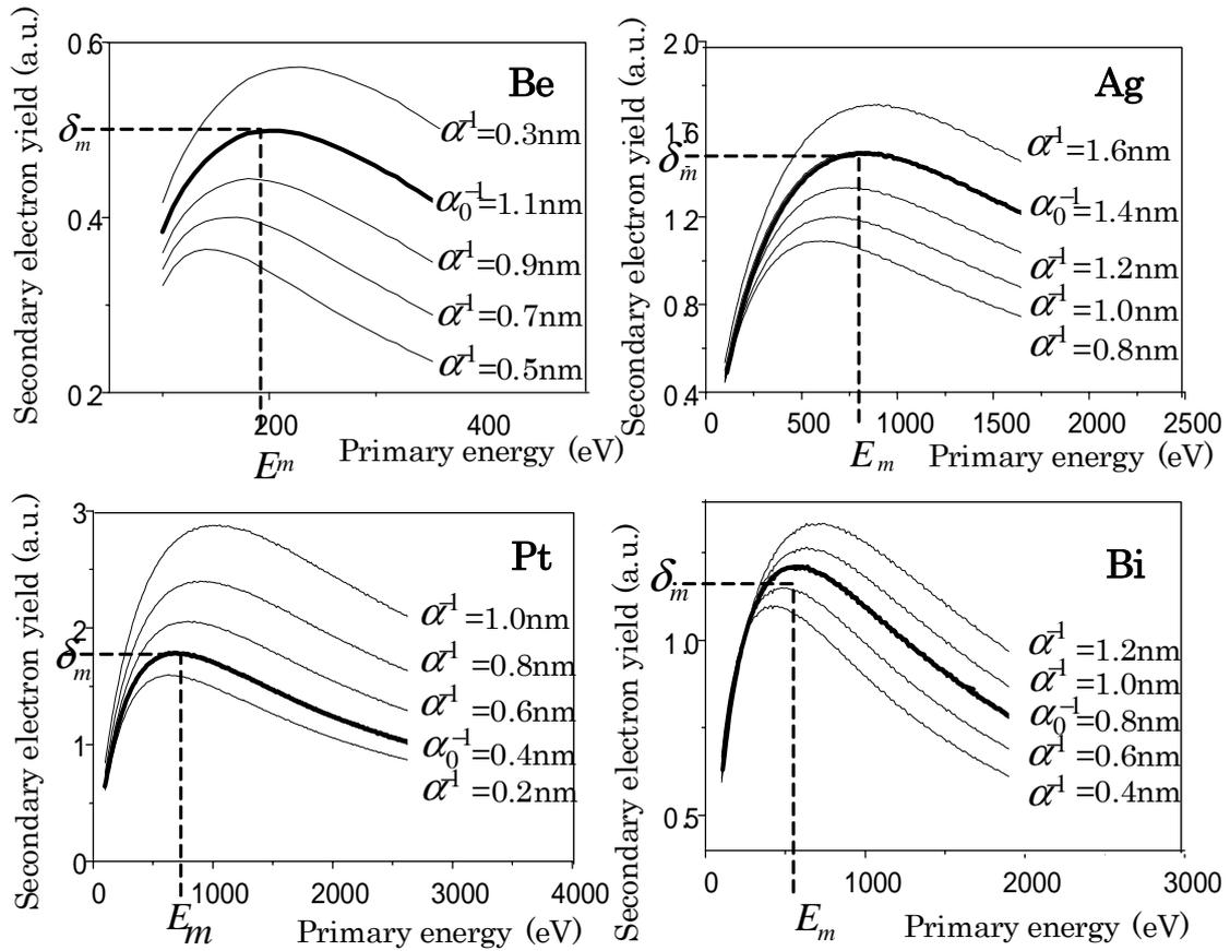
Fig.2 Theoretical  $\delta(E_p)$  obtained from Eq.4 for different values of absorption coefficient: (a)Be, (b)Ag, (c)Pt and (d)Bi.
